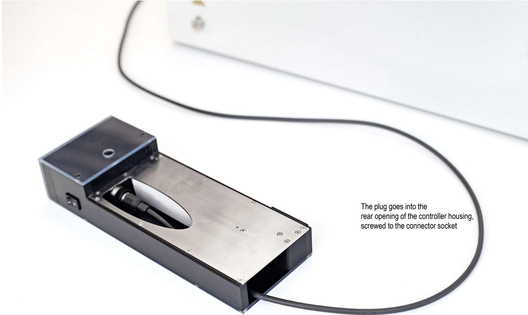
The plug goes into the rear opening of the controller housing, screwed to the connector socket
