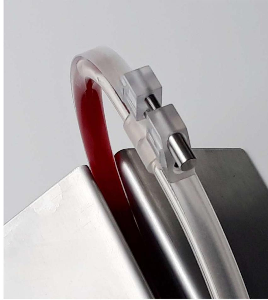
press the loop inside the tension ring
