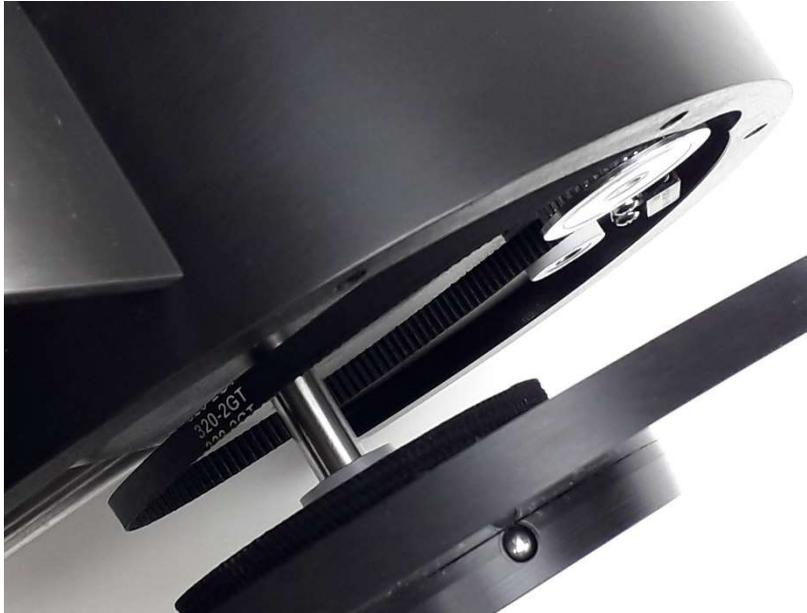
For renewed installation carefully lift the wheel on the axle with both hands. Gently push the drive belt onto the drive wheel with your fingertips by moving back and forth.
