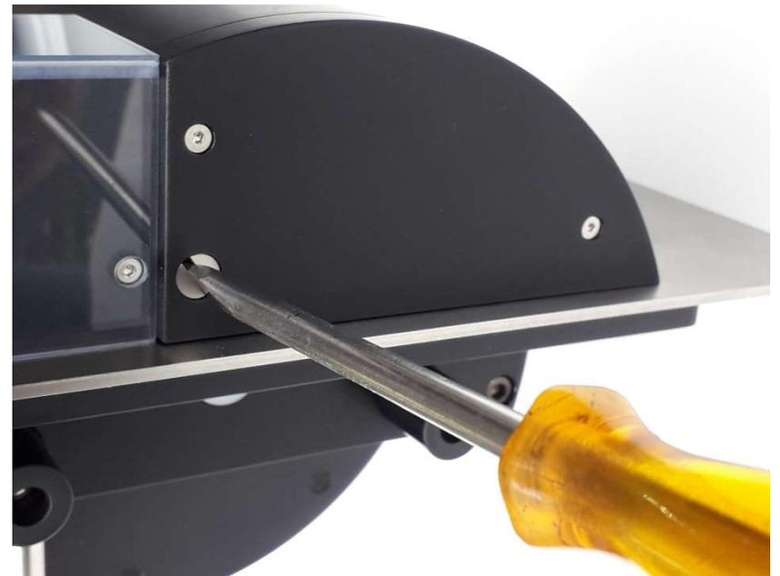
A small clockwise turn increases the belt tension
