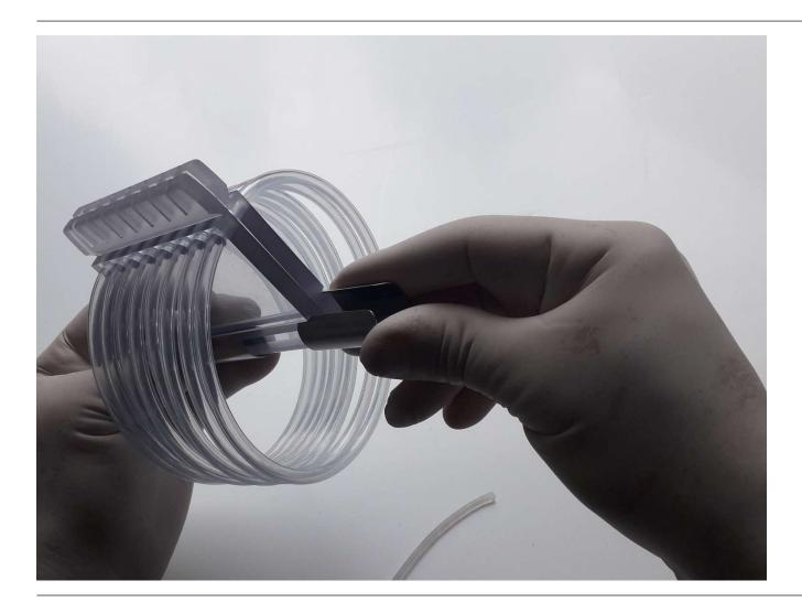
The clamping sleeves are inserted without tools and connect the 8-place tubing package into a handy unit.
