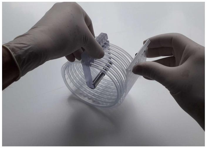
Putting on the plastic cover, the tubing rings arrange themselves automatically.
