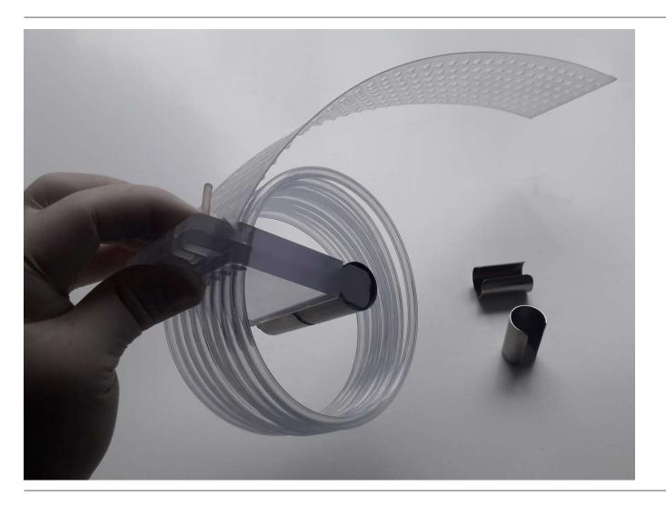
The plastic cover keeps the tubing rings in shape.
